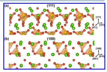
Figure 2. Side view of the C<sub>3</sub>S (a) (111) and (b) (100) surfaces.
