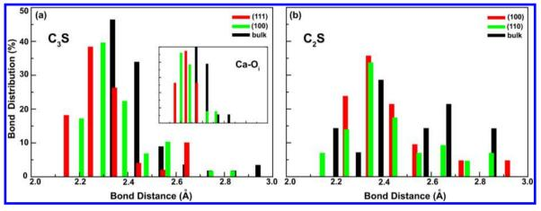
Figure 4. Ca-O bond distribution analysis of (a)  $C_3S$  (111) and (100) surfaces and  $C_3S$  bulk structure and (b)  $C_2S$  (100) and (110) surfaces and  $C_2S$  bulk structure. The inset shows  $C_3-O_3$  bond distribution of  $C_3S$ .
