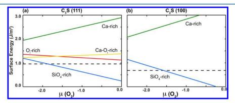
Figure 6. Surface energies of (a)  $C_3S$  (111) and (b)  $C_2S$  (100) as a function of oxygen chemical potential. The dashed lines denote stoichiometric surface energies.
