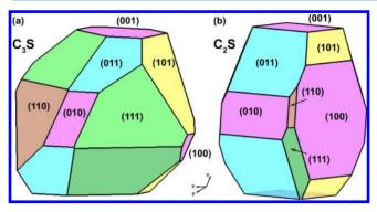
**Figure 5.** Wulff shapes of (a)  $C_3S$  and (b)  $C_2S$  based on the calculated surface energies for all low-index orientations (Table 1).
