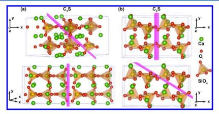
Figure 1. Relaxed crystal structure of (a)  $Ca_3SiO_5$  and (b)  $Ca_2SiO_4$  in two different orientations. The [111] and [100] planes for  $C_3S$  and [100] and [110] planes for  $C_2S$  are shown by pink planes. The Ca, O, and Si atoms are shown by green, red, and yellow spheres, respectively.
