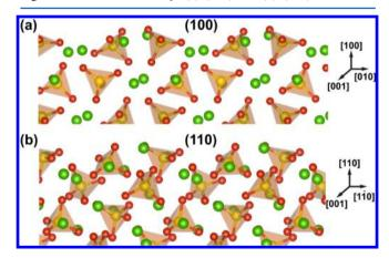
Figure 3. Side view of the  $C_2S$  (a) (100) and (b) (110) surfaces.
